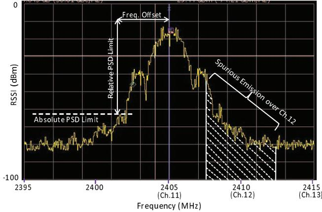
Fig. 10. Spurious Emission over Adjacent Channel (Center Ch. = 11)
