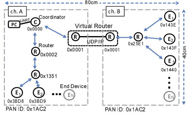
Fig. 9. Logical Structure of the Experiment
