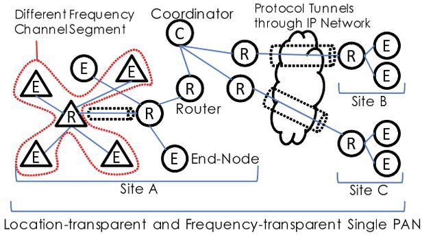
Fig. 2. Extending a PAN Domain over Multiple Frequency Channels and Different Locations with Protocol Tunneling
