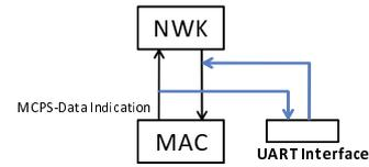
Fig. 3. Extraction/Insertion of Data Frames with MCPS Data Indication
