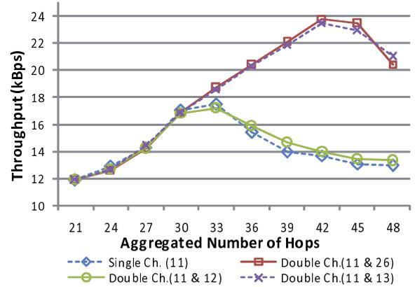
Fig. 11. Throughput Improvement of Splitting a Single-channel PAN into Double-channel Segments
