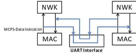
Fig. 4. Perpetual Exchange of MAC Frames between Two Nodes
