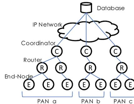
Fig. 1. Integration of Multiple ZigBee PANs
