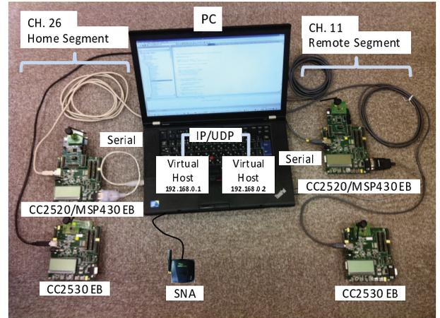
Fig. 7. Logical Structure of Implemented System
