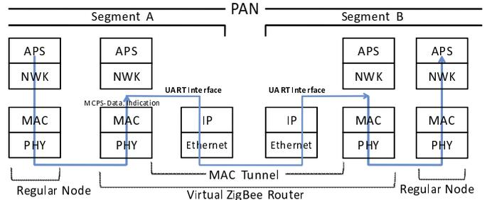
Fig. 5. Routing Packets through a MAC Tunnel between Segments
