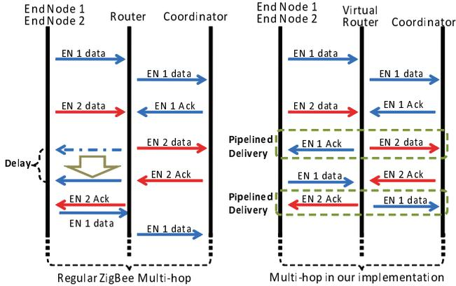
Fig. 6. Pipelined Data Multi-Hop by Virtual ZigBee Router
