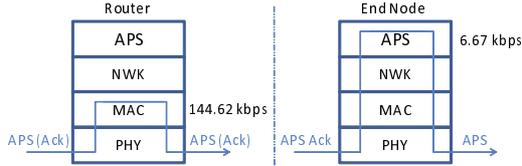
Fig. 8. Hardware Limit for APS and MAC Transaction
