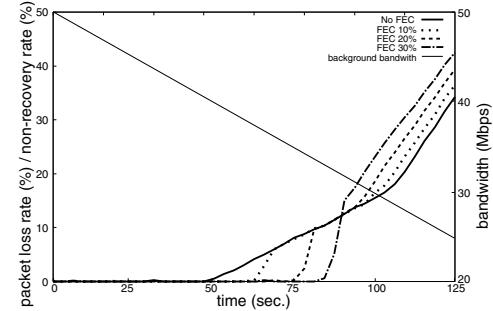
Fig. 2. Packet loss and non-recovery rate in full rate DVTS.
