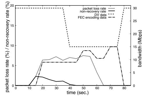
Fig. 8. Adaptive DVTS in the recovery of the network congestion
