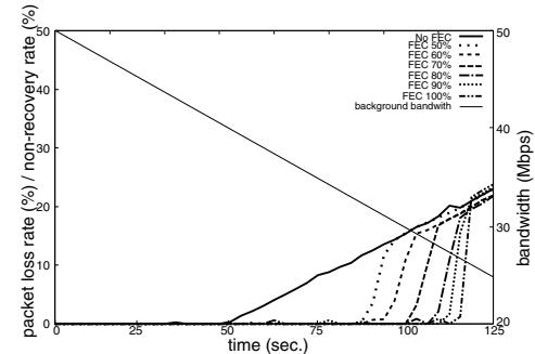
Fig. 3. Packet loss and non-recovery rate in half rate DVTS.
