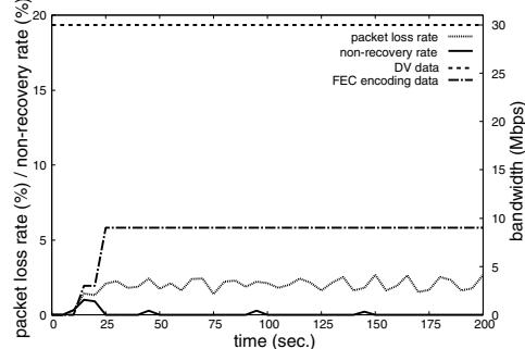
Fig. 5. Competition with normal DVTS flow over 100 Mbps link
