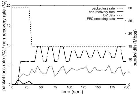
Fig. 7. Competition with normal DVTS flow over 90 Mbps link
