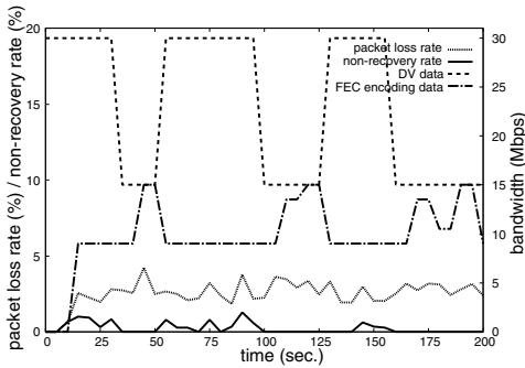
Fig. 6. Competition with normal DVTS flow over 95 Mbps link
