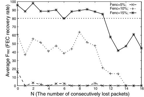
Fig. 1. The number of consecutively lost packet and FEC recovery rate.
